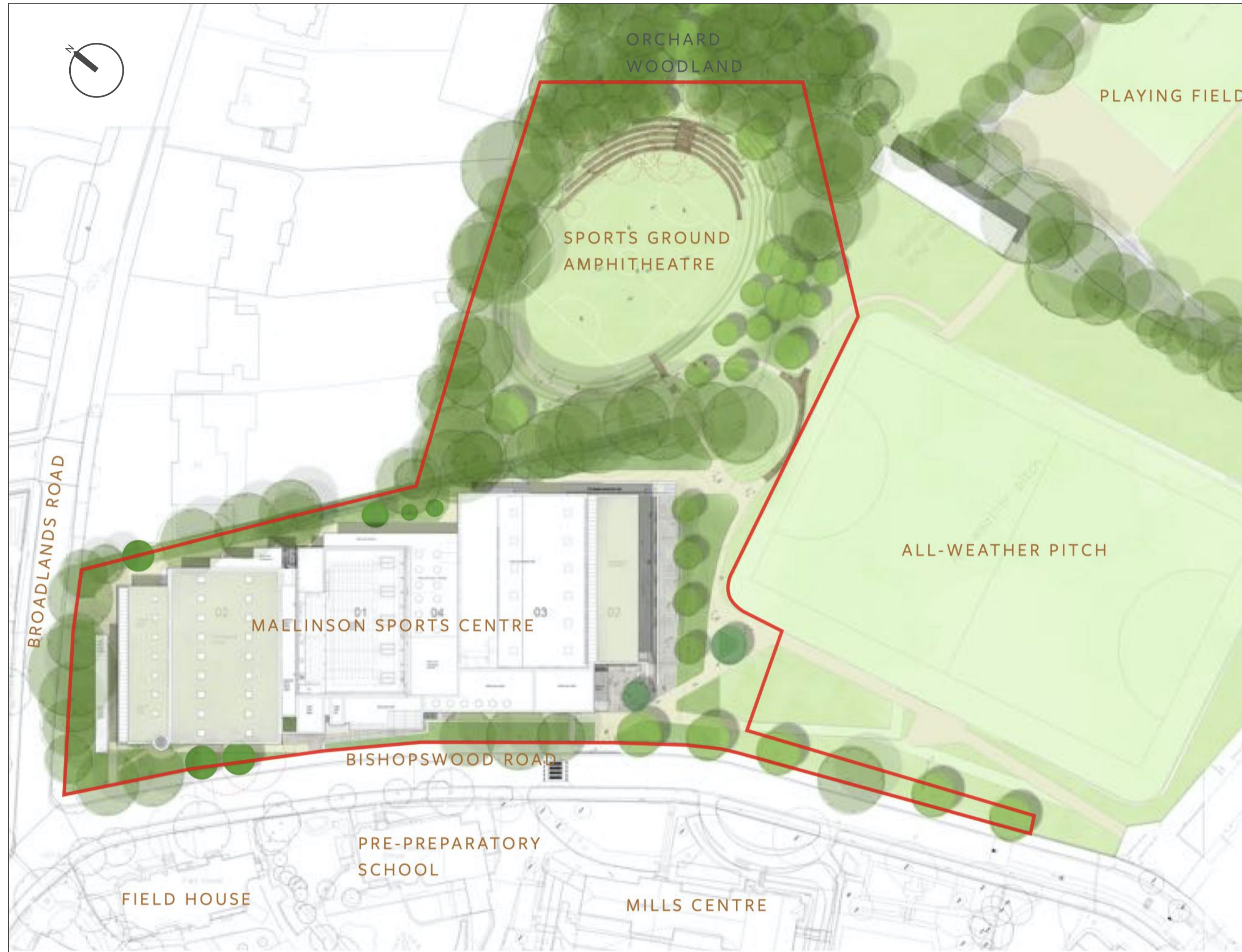
Site landscaping plan proposed, with perimeter trees and planting around MSC, Orchard sports pitch basin, and paths to outdoor sports pitches
